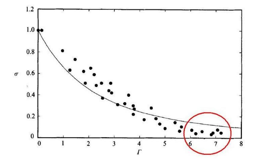
Foda&Cox's results<sup>7</sup> for an oil layer on water (experimental data points (•)) and a curve from the model equation of state (3) with  $\theta = 0.15$ .
